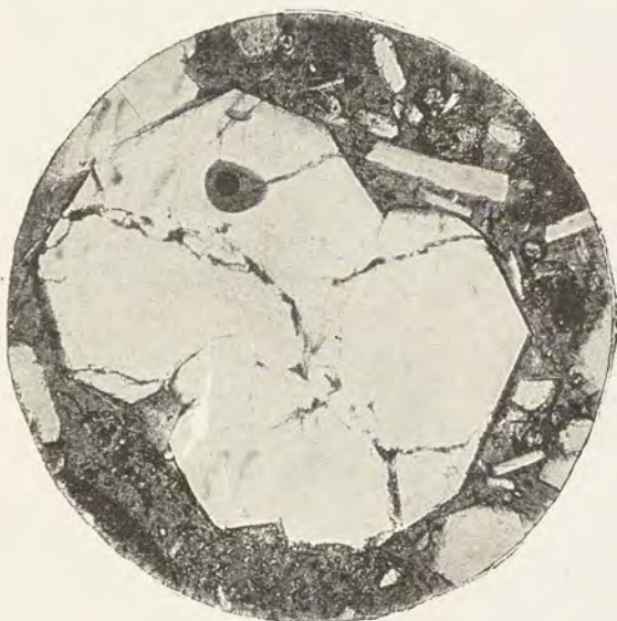
Fig. 96. Glassy enclosures in leucite. Lava from Vesuvius. Magnification 45.
